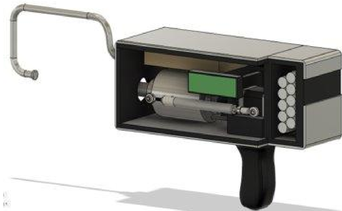
Figure 6-3. Device CAD Drawing: Full body with internal components shown
